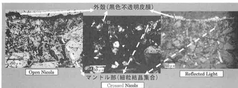
Photo.12 立堀風穴にある溶岩つらら石の縦断面の偏光顕微鏡写真(左側:オープンニコル、中央:クロスニコル、右側:反射像) Microphotographs (Left Side: Open Nicol, Middle: Crossed Nicol, Right Side: Reflected Light) of Longitudinal Section of Lava Stalactite Thin Section from Tachibori Fuketsu (Cave).
