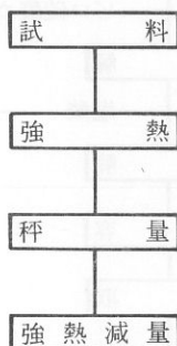
FIG. 9 無水硫酸 (SO 3 ) 定量方法の流れ図 The Flow Chart of Chemical Composition Analysis for SO 3
